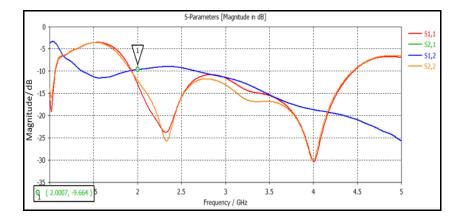
Figure 10. S-Parameter of vivaldi array antenna without metamaterial
