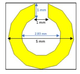
Figure 7. The size of ring metamaterial on vivaldi array antenna
