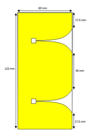
Figure 5. Vivaldi array antenna without metamaterial
