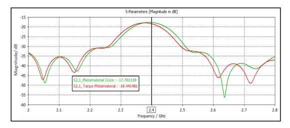
Figure 12. Comparison of mutual coupling between square array antenna without metamaterial and with ring metamaterial
