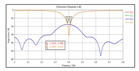
Figure 9. S-Parameter of square array antenna with ring metamaterial Metamaterial
