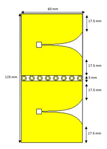
Figure 6. Vivaldi array antenna with ring metamaterial
