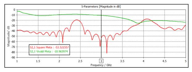
Figure 14. Comparison of Mutual Coupling between Square Array Antenna and Vivaldi Array Antenna using Ring Metamaterial
