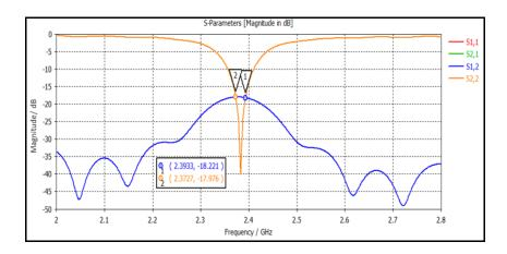
Figure 8. S-Parameter of square array antenna without metamaterial
