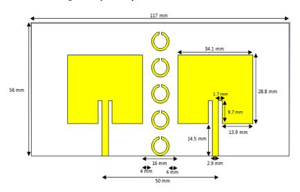
Figure 3. Square array antenna with ring metamaterial
