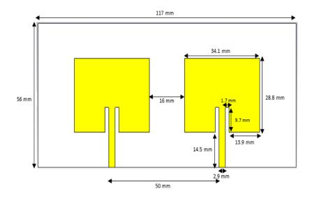
Figure 2. Square array antenna without metamaterial
