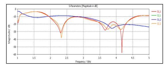
Figure 11. S-Parameter of Vivaldi Array Antenna with Ring Metamaterial
