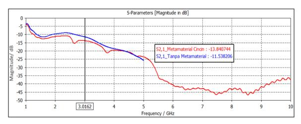
Figure 13. Comparison of mutual coupling between Vivaldi array antenna without metamaterial and with ring metamaterial
