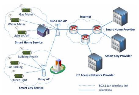
Figure 1. 802.11ah Network Model (Kim et.al., 2017)
