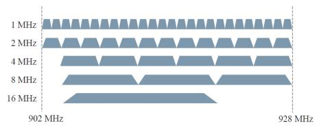
Figure 2. IEEE 802.11ah channelization (Sun et al., 2017)
