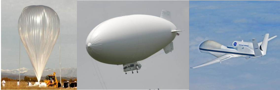
Gambar 2. Infrastruktur HAP (kiri-kanan): Balon, Airship , Aeroplane
